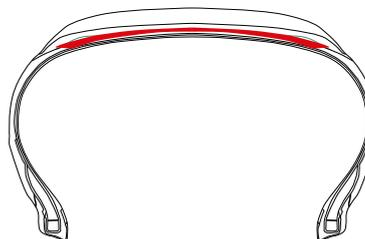
Low-heat-generating under tread, reduces energy-loss by sustaining rigidity.
