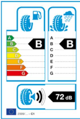
In 2012 the European Union introduced a tyre label, in order to provide standardised information on 3 specific performances; fuel efficiency, wet grip and external rolling noise.
